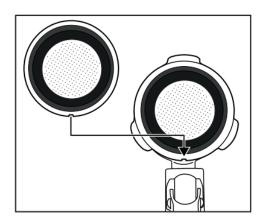
Rotate the filter slightly so that the tab secures the filter from falling out.
