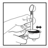
**Attention!** Too fine grinding or too much tamping can make it difficult for the water to pass through. If the water does not pass through the coffee filter, check the degree of grind you are using and also try not to grind the coffee too hard.
