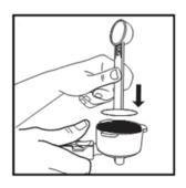
If the MAX mark on the filter is exceeded, remove the excess.
