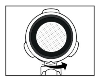
**Caution!** Do not remove the filter immediately after cooking until it has cooled!
